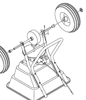
Install the left wheel (L) plus washer (G) on the outside of the wheel, secure the wheel with the hubcap (J).
