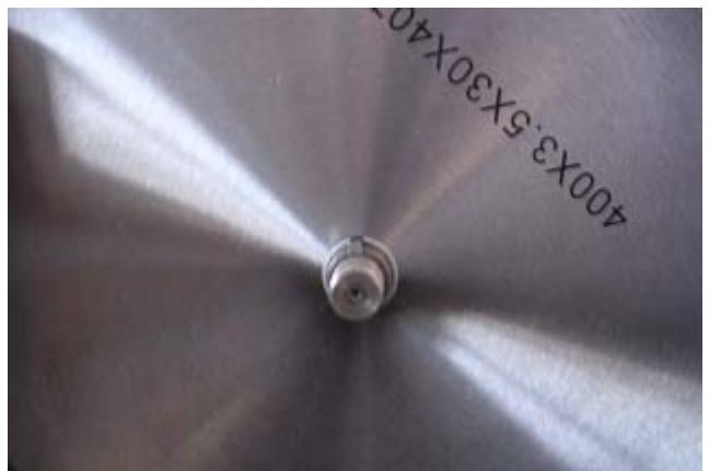
6. Put the outer flange of saw blade to the engine output shaft and screw the nut on.
