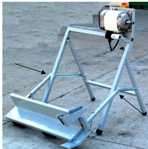
2. Uplift the holder "D" up like shown. At the same time, the protection shield "B" should be placed on the engine.
