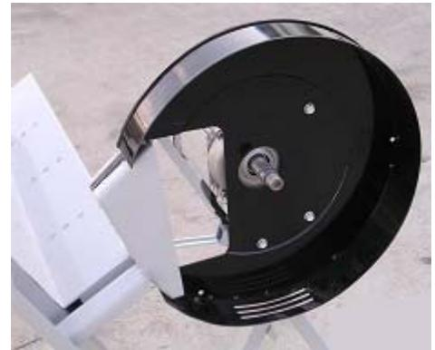
4. Put the inner flange of the blade saw to the engine output shaft
