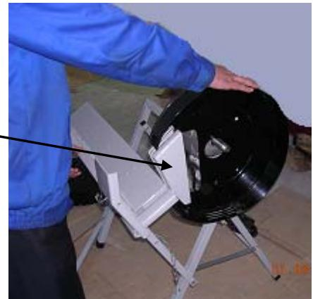
3. Fix the protection shield to the engine with the 3 bolts.
