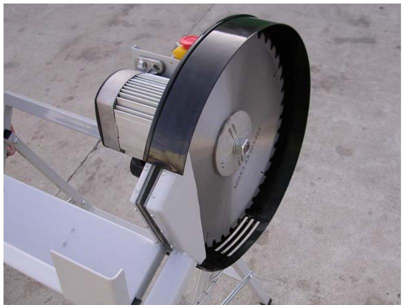
7. Fix the saw blade outer protection shield, using 3 long bolts.
