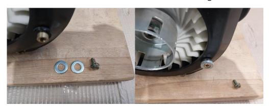
3. Mount the recoil starter with the 3 original bolts.
