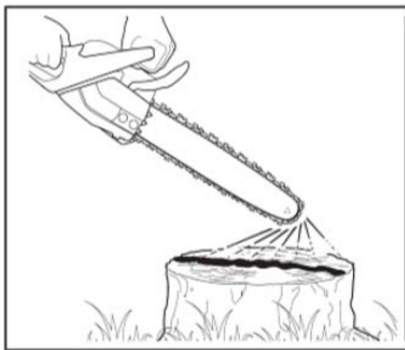
If no oil comes out, check that there is oil in oil tank and make sure the guide bar groove and holes are free from dirt. Also clean around the oil outlet behind the bar on machine.
